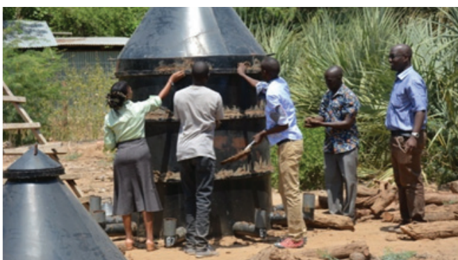
Environment officers in Turkana undergoing training on production of Prosopis charcoal using metal kiln
